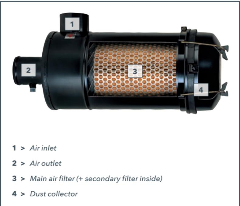
*The combustion air is thus routed through up to four filtering components including the prefilter. An effort that pays off, since WIRTGEN GROUP machines have to work perfectly under a wide range of different dustpolluted construction site conditions all over the world, which means each and every one of these elements has to be able to do its job with above-average efficiency.*
