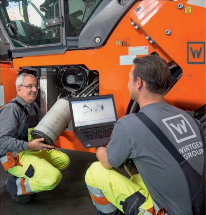
The **charge pressure filter** is directly at the outlet of the feed pump. It filters the hydraulic oil required before it is pumped into the circuit loop. Thus the hydraulic system is always supplied with the necessary quantity of oil.
