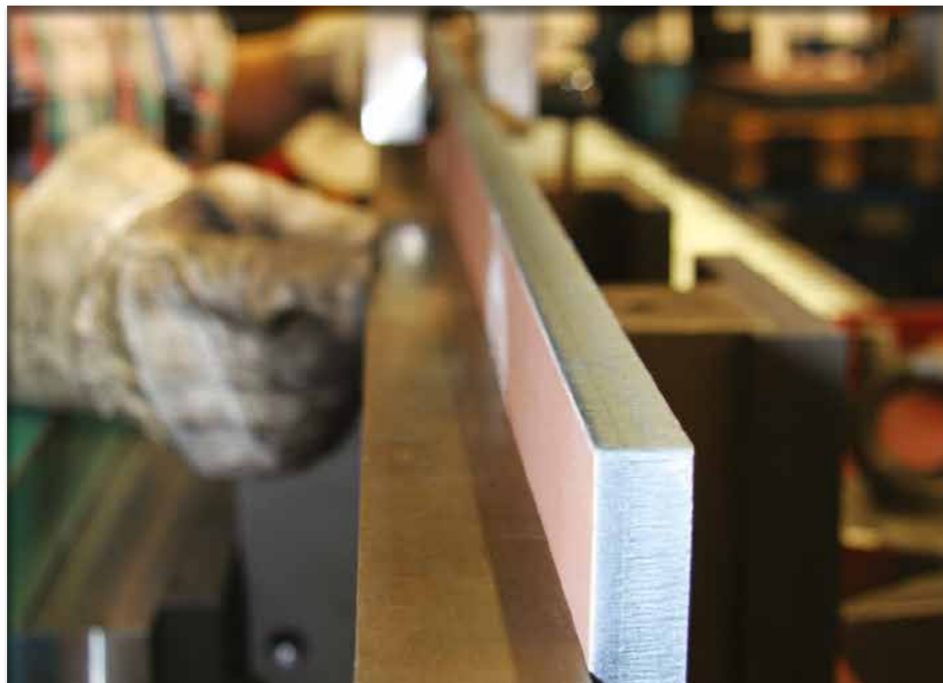
Tension-free alignment with an evenness error of max. 2/10 mm ensures a long service life, as the screed plate wears evenly.
