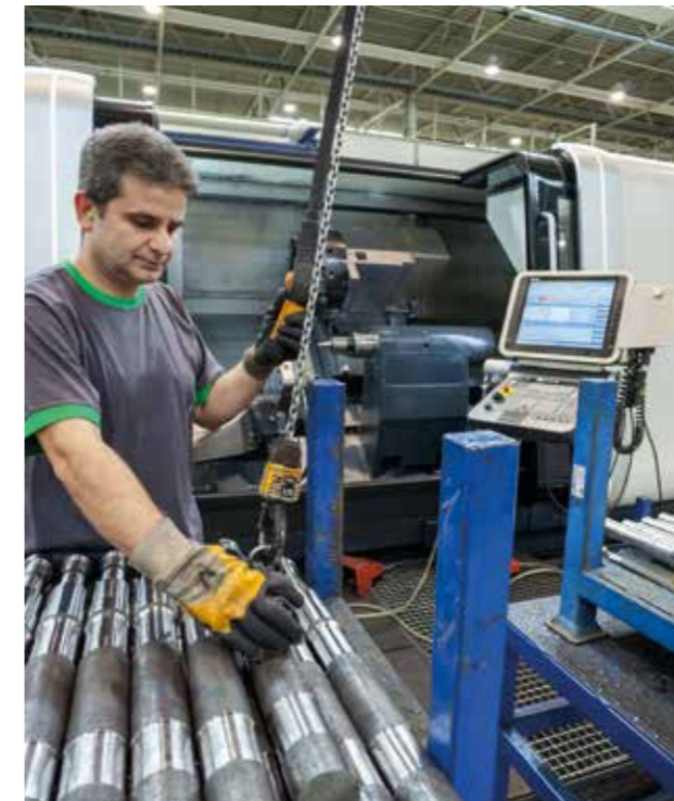
TOP LEFT: ..... Eccentric shafts for tamper drives.
