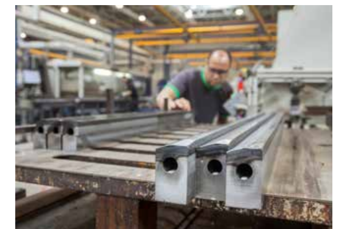
Tamper and pressure bar are hardened to a uniform depth of 5 mm.
