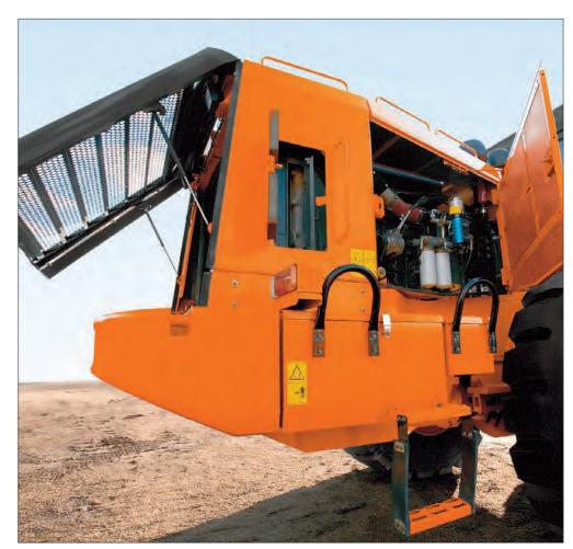
Easy Access to Engine and Filters Machine covers open wide for easy access to the engine and filters for efficient servicing and inspection. Filters and grease fittings are grouped for the convenience of replacement and lubrication.
