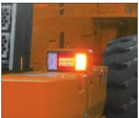
Front and rear working lights are bright halogen lamps for safer night-shift operation.
