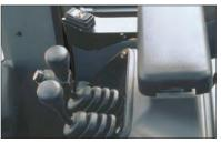
The directional switch is located next to control levers for easy travel direction changing. The operator does not need to left hand off the steering wheel.
