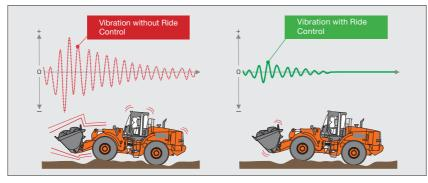
The ride control system can reduce pitching and bouncing when traveling on rough terrain and snow road. This system automatically controls the movement of machine to reduce shocks and vibration.
