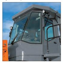
The cab gives good visibility with inside and outside rear view mirrors. The front windshield is a flat glass mounted with rubber gaskets for easy replacement. The cab rests on viscous mounting to absorb shocks and noise for operator comfort.
