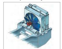
Hydraulic cooling fan speed varies with changes in operating temperatures to reduce noise and fuel consumption. The automatic reversible fan comes standard with a manual override that swings open for easy cleaning of radiators.
