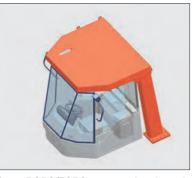
Outer ROPS/FOPS structure is adopted to protect the operator from injury in the case of an accident. ROPS: Roll-Over Protective Structure, ISO3471
