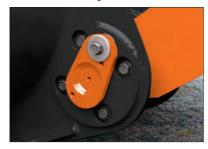
The bucket hinge pins are hermetically sealed to retain grease inside for longer service life.
