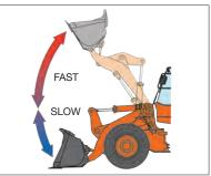
The Efficient Loading System (ELS) can increase traction force during digging while reducing fuel consumption. This achieves more production with less fuel.
