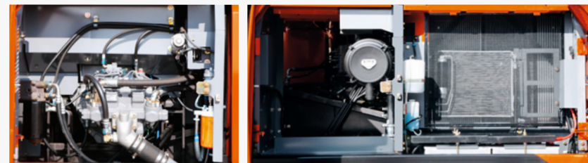
Grouped remote filters and inspection points
