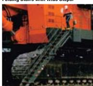
Folding stairs is designed for easy access to the machine for servicing and maintenance.
