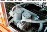
Hydraulic oil is filtered at high pressure to remove damage-causing contaminants. This filter is positioned down-line from the pumps to help prevent damage in the rare event of pump failure. Positioned for easy maintenance.
