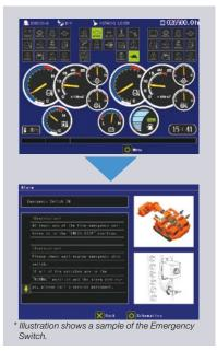
The operator can monitor machine conditions and operating status with a 10.5-inch color LCD. The controller provides instant fault diagnosis through all sensors, displaying warnings and countermeasures if failure arises.
