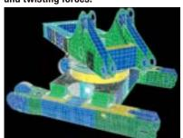
Computer-assisted analysis was used to check that the frame box can withstand heavy-duty excavation work.
