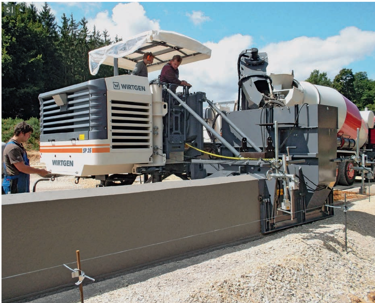
4-5 | The mould can be mounted on the left or right - modification is completed within an extremely short time.
