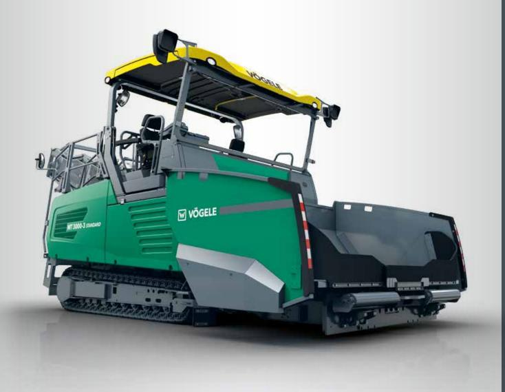
Maximum conveying capacity 1,200 t/h Conveyor 1.1 m wide Simple operation with ErgoPlus 3
